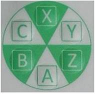
Select the Axis for JOG – Press the desired AXis
